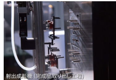
射出成形機 (完成品取り出し工程) Injection molding machine (Finished product exit process)
